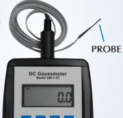
This simple instrument allows you to easily measure magnetic strength without any hassle. A new CESCO gaussmeter makes HACCP (Hazard Analysis Critical Control Points) compliance a snap. Place the probe at the maximum magnetism and read the meter. IT'S THAT EASY! It comes with everything you need: instructions, viewing paper that allows you to quickly locate the area of maximum magnetism, a replaceable 9V battery and a 48" flexible probe.
